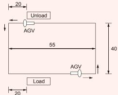
Considering a vehicle velocity of 50 m/min, availability of 0.95 and traffic factor of 0.9, the number of vehicles required to satisfy a demand of 50 delivery/hour is\_\_\_\_\_
