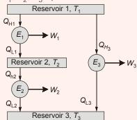
The efficiency of the engine  $E_3$  in terms of the efficiencies  $\eta_1$  and  $\eta_2$  of the engines  $E_1$ and  $E_2$ , respectively, is
