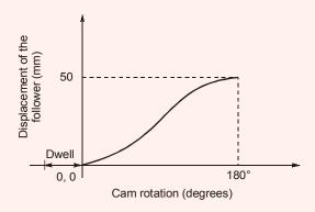
If the cam rotates at a uniform angular speed of 100 rpm. the speed of the follower (in mm/s) at the instance when the cam rotates 45° from the initial position is\_
