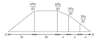
So,  $\theta_A - \theta_B$  is area of  $\frac{M}{EI}$  diagram between *A* and *B i.e.*
