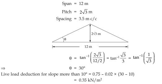
However as per IS875 (Part 2), minimum LL to be considered for design =  $0.4 \text{ kN/m}^2$ .
