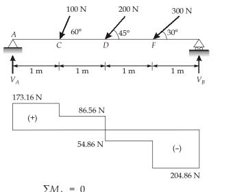
$$\Rightarrow \qquad 4 \times V_B = 300 \sin 30^\circ \times 3 + 200 \sin 45^\circ \times 2 + 100 \sin 60^\circ \times 1$$
