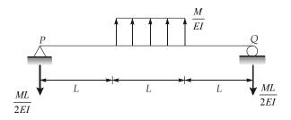
$\Delta_{\max}$  is the BM of conjugate beam and will occur at mid span.
