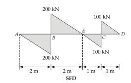
$(S.F)_{max} = 200 \text{ kN}$   $M_B = 100 \times 2 \times 1 = 200 \text{ kNm}$   $M_E = R_B \times 2 - 100 \times 4 \times 2 = 0$   $M_C = 100 \times 0.5 = 50 \text{ kNm}$  $(M)_{max} = 200 \text{ kNm}$
