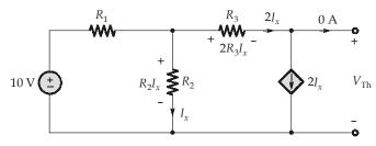
$$V_{\text{Th}} = -2R_3I_x + R_2I_x = (R_2 - 2R_3)I_x$$
