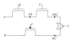
$Y = ABC + B\overline{C}$  [: The nodes acts as wired OR logic] =  $B(AC + \overline{C}) = B(A + \overline{C})$
