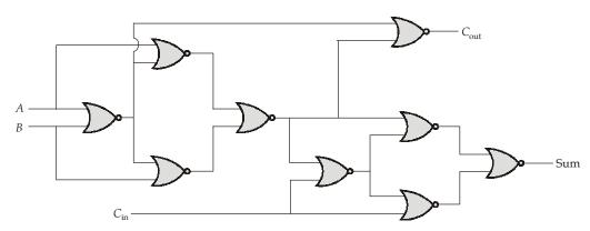
So, minimum 9 two-input NOR gates are required to design a full-adder circuit.
