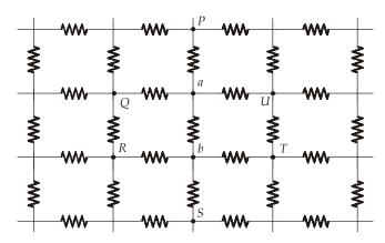
Let the current flowing into the circuit at the node 'a' will be I. Since the infinite network is symmetrical about 'a', the current I in going from 'a' to infinity, is divided equally along the branches aQ, aU, aP and ab as shown in the figure.
