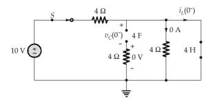
$$i_L(0^-) = \frac{10 \text{ V}}{4 \Omega} = 2.5 \text{ A}$$
