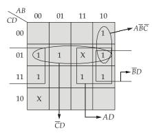
$$f(A, B, C, D) = \overline{C}D + AD + \overline{B}D + A\overline{B}\overline{C}$$
