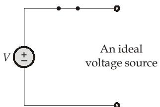
It is impossible to convert an ideal voltage source into its equivalent current source and hence the Norton's equivalent does not exist.
