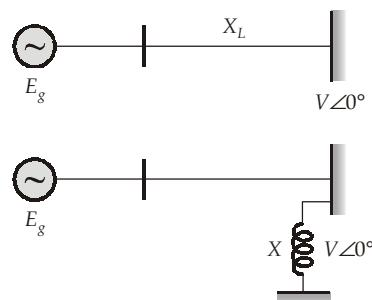
As the line reactance connecting the infinite bus and the generator remains unaffected after connecting the shunt reactor at the infinite bus therefore, the stability limit  $\left(\frac{V_{Eg}}{X_L}\right)$  remains constant.
