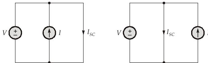
Since the violation of KVL in the circuit physical connection is not possible and hence it's impossible to evaluate  $I_{SC}$ , so the Norton's equivalent does not exist.
