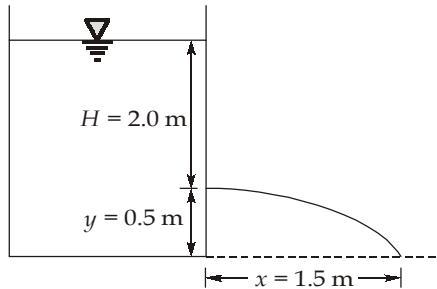
Coefficient of velocity,  $C_v = \frac{x}{2\sqrt{yH}} = \frac{1.5}{2\sqrt{0.5 \times 2.0}} = 0.75$
