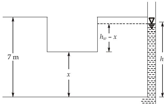
At  $x_1 = 3 \text{ m}$ , quick sand condition,  $h_{w1} = ?$
