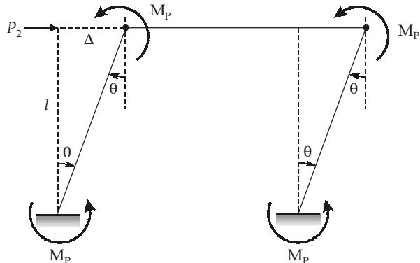
Applying principle of virtual work.
