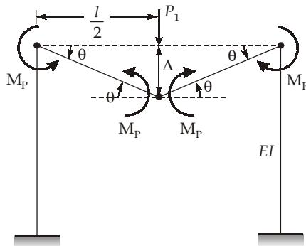
Applying principle of virtual work.
