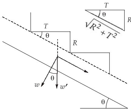
$w$  = Weight of slab per  $\text{m}^2$  at right angle to the direction of flight
