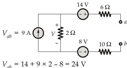
$$V_{ab} = 14 + 9 \times 2 - 8 = 24 \text{ V}$$
