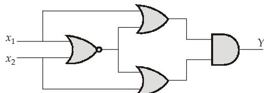
$$Y = (X_1 + \overline{X_1} \cdot \overline{X_2}) \cdot (X_2 + \overline{X_1} \cdot \overline{X_2})$$
