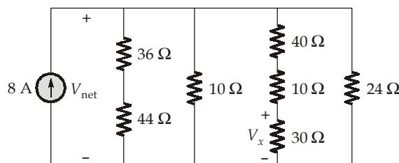
The voltage across the 8 A current source is equal to
