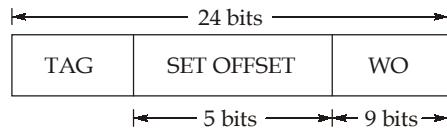
$$\begin{aligned} \text{Main memory size} &= 32768 \times 512 \\ &= 2^{15} \times 2^9 = 2^{24} \text{ bytes} \end{aligned}$$
