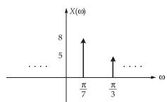
The frequency components in the spectrum are integer multiples of the fundamental frequency  $\omega_0$ . Thus, the fundamental frequency,
