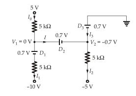
$$I_0 = \frac{5 \text{ V} - 0 \text{ V}}{5 \text{ k}\Omega} = 1 \text{ mA}$$
