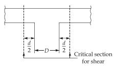
The critical section for punching shear in a flat slab is located at a distance of d/2 (half the effective depth) from the face of the column.
