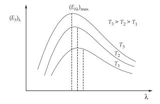
$(E_{b\lambda})_{\text{max}}$ : Maximum monochromatic emissive power
