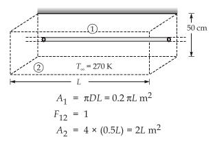
For radiative heat transfer coefficient of surface (2),
