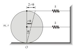
Equation of motion for pure rotation about point 'O'
