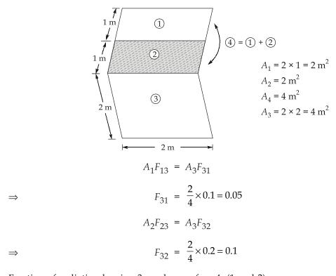
Fraction of radiation leaving 3 reaches surface 4, (1 and 2)
