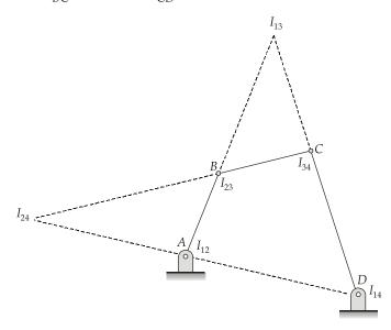
As  $I_{23}$  lies in between AB and BC so links AB and BC rotate in opposite direction. Similarly  $I_{34}$  lies in between BC and CD so links BC and CD rotate in opposite direction.
