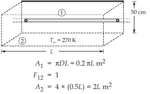
$$Q_{12} = F_{12}A_1\sigma(T_1^4 - T_2^4)$$
