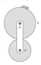
$$\frac{\omega_S - \omega_A}{\omega_P - \omega_A} = -\frac{R_P}{R_S}$$
