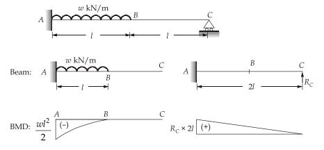
The moment of  $\frac{M}{EI}$  diagram between A and C about C is zero as deflection at C is zero.
