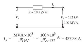
Transmission loss  $(P_L) = 3 \times I_R^2 R = 3 \times (437.38)^2 \times 10 = 5.73 \text{ MW}$
