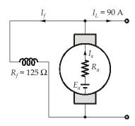
$$E = \frac{P\phi NZ}{60 \text{ A}} = \frac{4 \times 0.1 \times 1000 \times 300}{60 \times 4} = 500 \text{ V}$$
