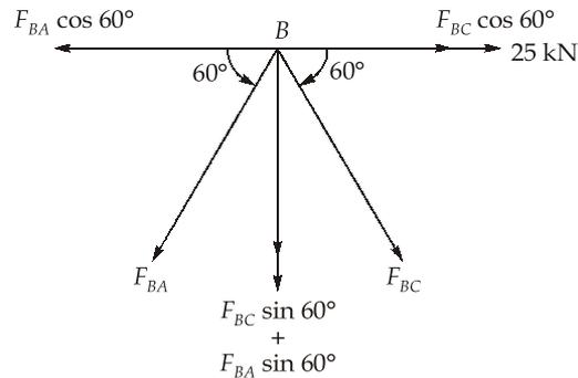
$$\begin{aligned} \Rightarrow \quad \Sigma f_y &= 0 \\ F_{BC} \sin 60^\circ + F_{BA} \sin 60^\circ &= 0 \\ F_{BC} &= -F_{BA} \quad \dots(i) \\ \Sigma f_x &= 0 \\ F_{BA} \cos 60^\circ &= F_{BC} \cos 60^\circ + 25 \\ F_{BA} \left(\frac{1}{2}\right) &= -F_{BA} \left(\frac{1}{2}\right) + 25 \\ F_{BA} &= 25 \text{ kN (tensile)} \end{aligned}$$
