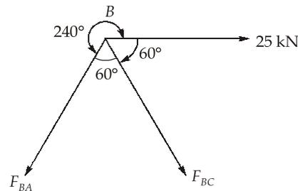
$$\begin{aligned} \Rightarrow \quad \frac{F_{BA}}{\sin 60^\circ} &= \frac{25}{\sin 60^\circ} \\ \Rightarrow \quad F_{BA} &= 25 \text{ kN (tensile)} \end{aligned}$$
