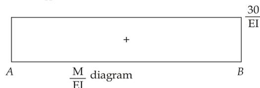
$$\Delta_A = t_{BA} = \text{Deflection at B with respect to tangent at A}$$
