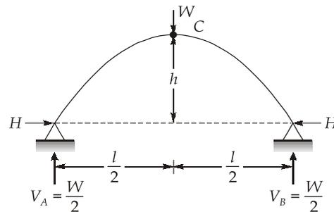
Vertical support reaction,  $V_A = V_B = \frac{W}{2}$
