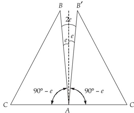
By reversing the instrument or part of it, the error becomes apparent. The magnitude of apparent error is double the true error because the reversion simply places the error as much to one side as it was to the opposite side before reversion.
