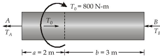
The fixing couple  $T_A$  and  $T_B$  at A and B respectively are given by
