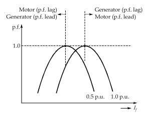
From the diagram above shown if  $I_f$  increases then power factor decreases when generator operates on lagging power factor.
