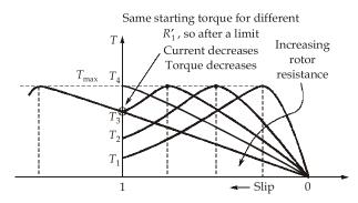
As R increases, starting torque increases upto maximum torque  $(T_4 = T_{\text{max}} > T_3 > T_2 > T_1)$  but rotor consumes more power so copper loss increases and efficiency decreases.
