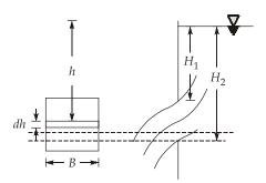
Discharge through elemental strip =  $c_d$  (Area) × Velocity =  $c_d (Bdh) \sqrt{2gh}$
