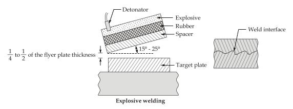
The minimum distance between the two plates is of the order of  $\frac{1}{4}$  to  $\frac{1}{2}$  of the flyer plate thickness.
