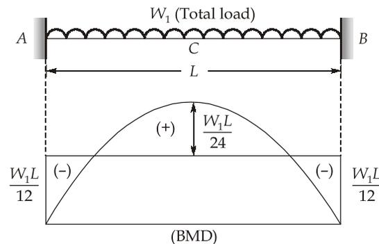
$\therefore$   $BM \text{ at } A > BM \text{ at } C$
