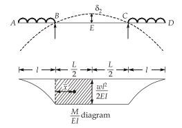
$\bar{x} = \frac{L}{4}$ Here, Shaded area =  $\frac{wl^2}{2EI} \times \frac{L}{2}$  $\delta_2 = A\overline{x} = \frac{wl^2}{2FI} \times \frac{L}{2} \times \frac{L}{4}$ :.
