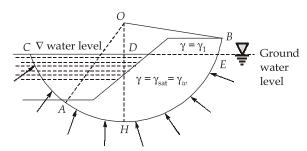
From the figure, it can be seen that the body of water in the half segment CDH balances that of the water contained in the other half segment DEH. The moments of the water pressure balance each other.
