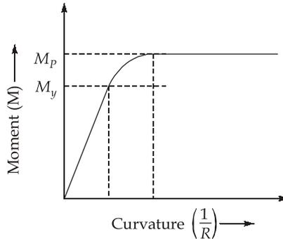
From the graph it is clear that at the location of plastic hinge developed in a structure, curvature is infinite
