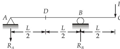
$$\begin{aligned} \Sigma F_y = 0, \\ \Rightarrow R_B - R_A = P \end{aligned}$$
