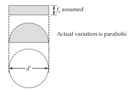
Distribution of direct stress on the portion of plate between the bolt holes is assumed to be constant.
