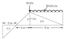
ILD for BM at C Maximum bending moment at *C*,
