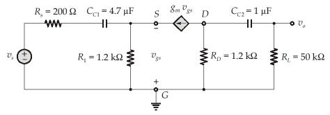
Calculation of time constant ( $\tau_1$ ) associated with  $C_{C1}$ :
