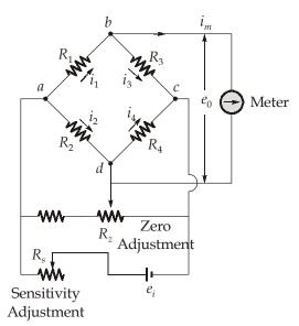
For measurement of rapidly changing input signals, the deflection type bridge is used. When the input changes, the resistance  $R_1$  changes producing an unbalance causing a voltage to appear across the meter. The deflection of meter is indicative of the value of resistance and the scale of the meter may be calibrated to read the value of resistance directly.
