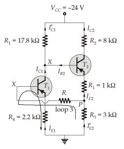
Applying KVL of collector-emitter loop for transistor  $T_{\rm 1}$  we get,
