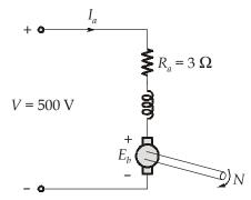
Mechanical power developed =  $E_b I_a$  = 4000 W
