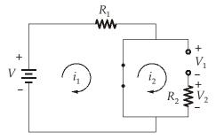
Let the clockwise mesh current be  $i_1$  and  $i_2$ . At  $t = 0^+$  the mesh equations are,
