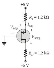
By assuming that the transistor is in saturation mode and taking the numerical values of  $I_{DQ}$  in mA units, we get,
