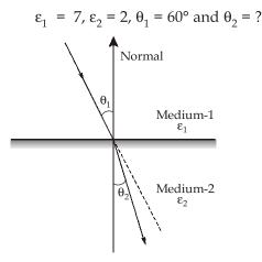
The tangential components of the electric field is continuous,
