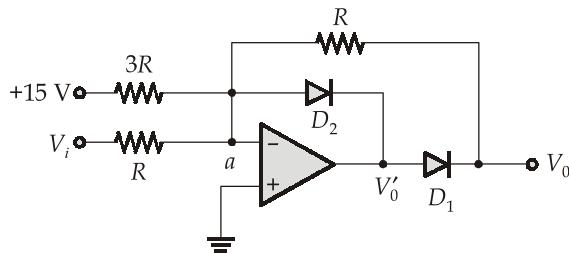
During a portion of negative cycle  $V'_o$  can become positive. Then  $D_1$  conducts and  $D_2$  becomes off. Only then circuit provides a non-zero output  $V_o$ .
