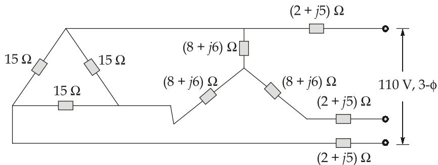
Convert  $\Delta$  to equivalent  $\gamma$  having  $\frac{15}{3} = 5\Omega$  per phase
