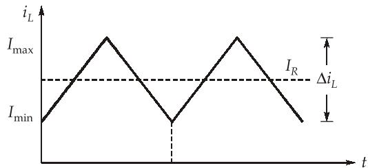
$$I_{\max} = I_L + \frac{\Delta i_L}{2} = V_0 \left( \frac{1}{R} + \frac{1-D}{2Lf} \right)$$
