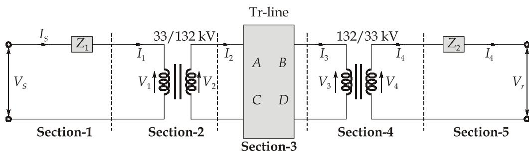
$$V_4 = V_r + Z_2 I_r; \quad I_4 = I_r$$
