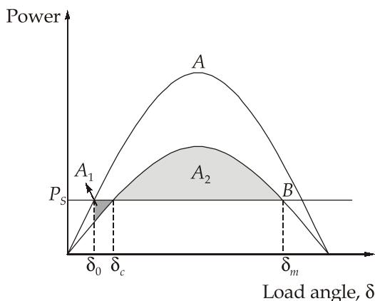
$$\text{Steady state power limit, } P_{\max} = \frac{EV}{X} = \frac{1.2 \times 1}{0.522} = 2.298 \text{ pu}$$
