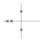
$2(s^2 + 1)(s^2 + 1) = 0 \Rightarrow s = \pm j$ . Hence, multiple poles exist on imaginary axis at  $s = \pm j$ . Therefore, the system is unstable and thus, the gain margin is not positive.
