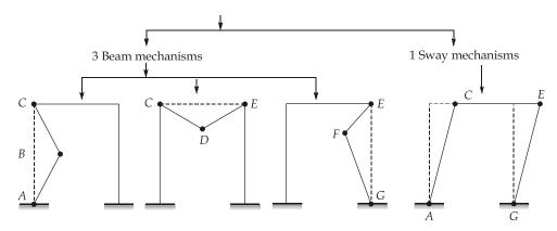
**NOTE**: Combined mechanism is a dependent mechanism, which depends upon beam and sway mechanisms.
