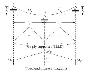
$$M_A\left(\frac{l_1}{I_1}\right) + 2M_B\left(\frac{l_1}{I_1} + \frac{l_2}{I_2}\right) + M_C\left(\frac{l_2}{I_2}\right) = -6\left(\frac{A_1\overline{x}_1}{I_1l_1} + \frac{A_2\overline{x}_2}{I_2l_2}\right) + 6E\left(\frac{\delta_1}{l_1} + \frac{\delta_2}{l_2}\right)$$
