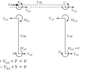
$$\Sigma F_{x} = 0 \implies V_{BA} + V_{CD} + P = 0$$
