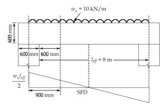
Distance from center of support  $(d') = 600 + \frac{600}{2} = 900 \text{ mm}$
