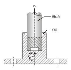
Radius of shaft and recess,  $R_i = 0.6 R_o$
