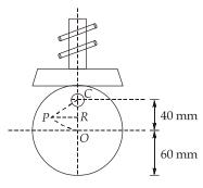
Given : e = 40 mm; m = 3 kg; s = 5 N/mm = 5000 N/m; P = 60 N +  $mg = 60 + 3 \times 9.81$ Speed at which the follower begins to lift from the cam surface or the jump speed is
