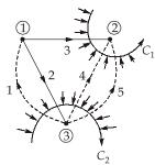
In the figure shown,  $C_1$  and  $C_2$  are fundamental cut-sets. We take the matrix element as +1 when the corresponding branch is oriented in the same direction as cut-set. Otherwise the element is -1 when the orientation of the cut-set and branch is opposite.
