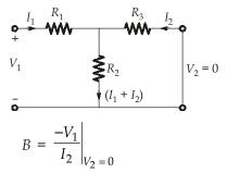
To obtain the parameter 'B', short-circuit the output port i.e.  $V_2 = 0$ . Applying KVL to input-port,
