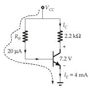
On applying KVL in the base emitter loop, we get,
