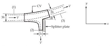
As the weight of water and friction along plate is neglected, so the force by jet on the plate in *y*-direction must be zero.
