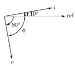
As  $\phi = 90^{\circ}$  and *i* leads *V*, it implies that the element is capacitor.
