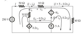
Applying KVL around the outer loop,
