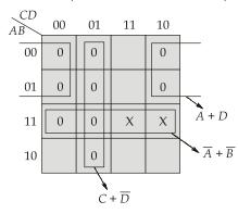
$$f = (A+D)(\overline{A}+\overline{B})(C+\overline{D})$$
