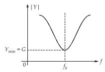
Since net admittance is minimum, the net impedance is maximum and purely resistive. Thus, the current is minimum and in phase with the applied voltage.
