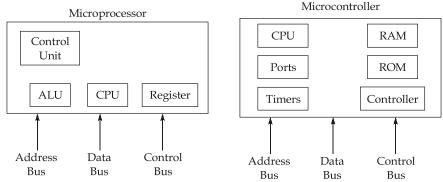
Microcontrollers are designed for embedded applications where reliability and fault tolerance
