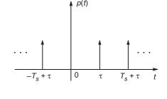
$$\Rightarrow P(\omega) = 2\pi \sum_{n=-\infty}^{\infty} C_n \delta(\omega - n\omega_s) = 2\pi \sum_{n=-\infty}^{\infty} \frac{e^{-jn\omega_s \tau}}{T_s} \delta(\omega - n\omega_s)$$
