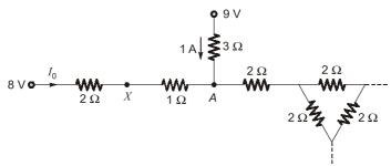
Voltage at node A is =  $9 - (3 \times 1) = 6 \text{ V}$
