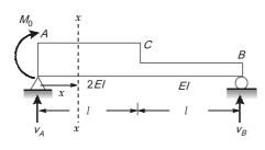
Let  $V_{\rm A}$  and  $V_{\rm B}$  be the vertical reactions at A and B respectively.
