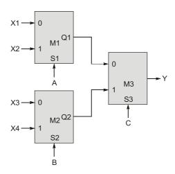
For an instance of inputs X1 = 1, X2 = 1, X3 = 0, and X4 = 0, the number of combinations of A, B, C that give the output Y = 1 is \_\_\_\_\_.
