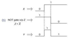
Output *Y* is logic 1 for small time interval whenever *X* changes from logic '0' to logic '1', assuming gates are having some delay.
