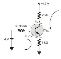
$$V_{\text{Th}} = \frac{12 \times 50k}{150k} = 4 \text{ V}$$
