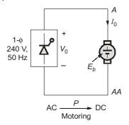
Rating of DC machine 210 V, 10 A, 1200 rpm,
