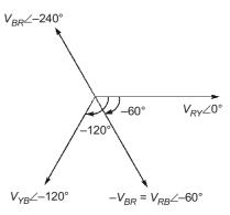
$$V_{RY} = 400 \angle 0^{\circ}$$
