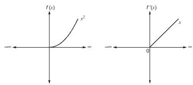
$\therefore$  f(x) is differential and f'(x) is continuous but f''(x) is not continuous.
