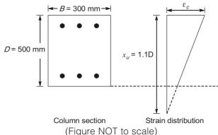
The maximum compressive strain ( $\varepsilon_c$ ) at highly compressive extreme fiber in concrete,
