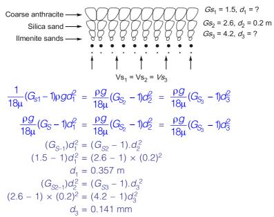
**NOTE**: The logic is that if we are creating 3 layers for better filtration and if we want those layers to be intact, even after backwashing, then we need to ensure that as the backwashing is stopped, each layer settles with the same velocity so that the stratification is maintained as it is.
