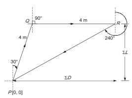
Horizontal distance of traverse from P to  $R = \Sigma D$
