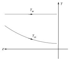
The rate of increase in bulk mean temperature along the flow  $\left(\frac{dT_m}{dz}\right)$  increase exponentially along the flow direction (z).
