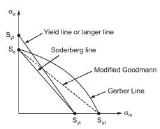
Soderberg line is the most conservative fatigue failure criterion.
