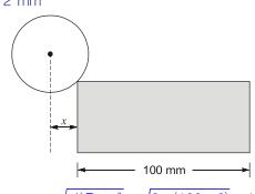
Approach length,  $x = \sqrt{d(D-d)} = \sqrt{2 \times (100-2)} = 14 \text{ mm}$
