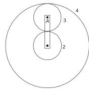
Given:  $T_2 = 19$ ,  $T_3 = 24$ ,  $N_4 = 0$ ,  $N_4 = 20$  rpm (CCW)
