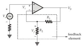
Feedback element is directly connected to the output, therefore voltage sampling. Feedback element is not directly connected to the input, therefore series mixing. The feedback present in above configuration is voltage series.
