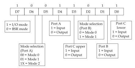
To configure 8255 to operate in Mode 0 with all ports as input ports, the control world would be 1001 1011 = 9B H.
