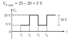
Difference of  $V_{0\text{max}}$  and  $V_{0\text{min}}$  = 35 - 5 = 30 V
