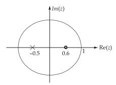
[As the filter is causal, the ROC of the impulse repsonse must be right sided] Since ROC includes the unit circle, hence the system is stable.
