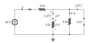
$$\begin{split} i_L(0^-) &= \frac{10 \text{ V}}{4 \,\Omega} = 2.5 \text{ A} \\ v_C(0^-) &= 0 \text{ V} \\ v_C(0^+) &= v_C(0^-) = 0 \text{ V} \\ i_L(0^+) &= i_L(0^-) = 2.5 \text{ A} \\ v_L(0^+) &= -(4 \,\Omega) \frac{i_L(0^+)}{2} \\ &= -4 \times \frac{2.5}{2} = -5 \text{ V} \end{split}$$
