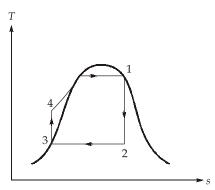
Given :  $h_1$  = 2785 kJ/kg;  $h_2$  = 1863 kJ/kg;  $h_3$  = 192 kJ/kg;  $h_4$  = 198 kJ/kg
