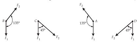
The resultant of  $\vec{F}_1$  and  $\vec{F}_2$  is maximum for rivet C and D, as they are at 45° of inclination with each other. Hence C and D rivets are the most loaded rivet.
