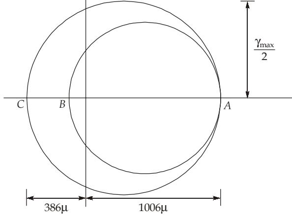
(c) Maximum shear strain,  $\gamma_{max}$ ,
