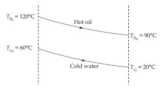
Counter flow heat exchanger
