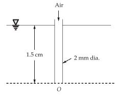
Pressure inside the bubble =  $200 \text{ N/m}^2$
