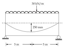
Intensity of equivalent load due to prestress,
