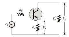
$$\beta = \text{Feedback factor} = \frac{-I_C R_E}{I_C R_C} = \frac{-R_E}{R_C}$$
