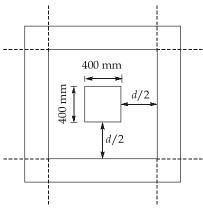
The critical section is taken at a distance  $\frac{d}{2}$  from face of column
