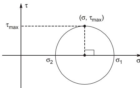
Since the plane of maximum shear stress is at inclination of  $90^\circ$  to principal plane in Mohr's circle.
