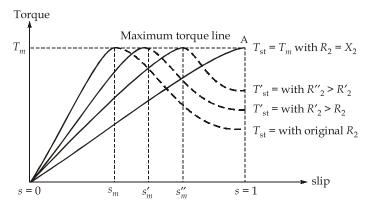
Hence, starting torque increases with increase in rotor resistance. But it also causes more rotor losses, hence efficiency decreases.
