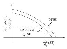
For same probability of error, QPSK and BPSK requires less  $\frac{E_b}{N_0}$  than DPSK.
