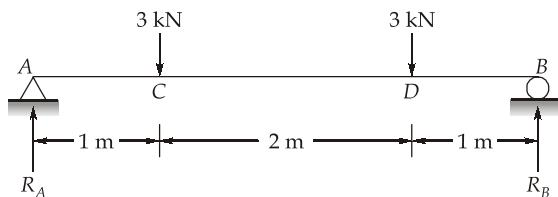
As the load on the beam is symmetrical, reactions  $R_A$  and  $R_B$  are equal
