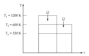
$$\text{Loss of available energy, } I = T_o (\Delta S)_{\text{uni}}$$
