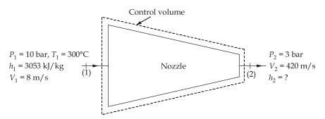
Applying steady flow energy equation on the control volume,
