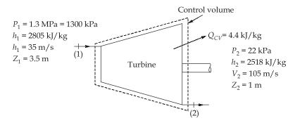
Applying steady flow energy equation on the control volume, we get,
