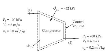
Applying steady flow energy equation on the control volume, we get,
