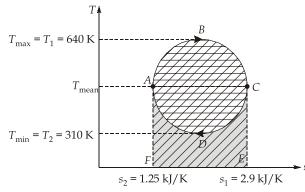
$$T_{\text{mean}} = \frac{T_1 + T_2}{2} = \frac{640 + 310}{2} = 475 \text{ K}$$
