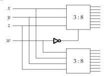
Two 3:8 decoders and an inverter are required to implement 4:16 decoder.
