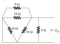
$$R_{\text{th}} = 9 \parallel [(9 \parallel 18) \parallel 18] = 9 \parallel \frac{9}{2} = \frac{9 \times \frac{9}{2}}{9 + \frac{9}{2}} = \frac{9 \times 9}{27} = 3 \Omega$$
