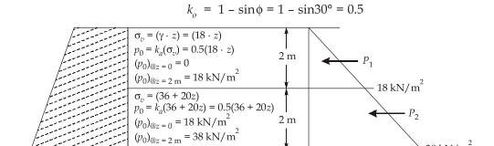
• Total lateral earth pressure at rest is given as
