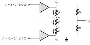
$$V_{o_1} = IR + V_1$$
