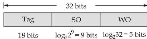
$$\begin{aligned} \text{Tag memory size} &= S \times P \times \# \text{ tag bits} \\ &= 2^9 \times 4 \times (18 + 1 + 1 + 2) = 2^9 \times 2^2 \times 22 \text{ bits} \\ &= 2^{10} \times 2 \times 22 \text{ bits} = 44 \text{ K bits} \end{aligned}$$
