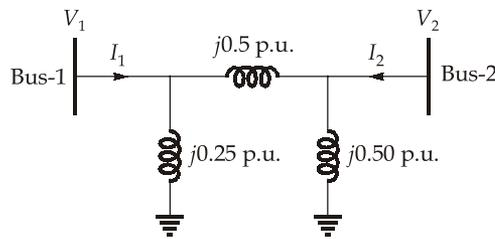
$$\begin{aligned} Z_{11} &= \left. \frac{V_1}{I_1} \right|_{I_2=0} = j0.25 \parallel (j0.50 + j0.50) \\ &= (j0.25 \parallel j1) = j \frac{1 \times 0.25}{1.25} = j0.20 \text{ p.u.} \end{aligned}$$
