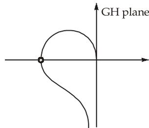
$$\begin{aligned} \text{P.M.} &= 180^\circ + \phi|_{\omega_{gc}} \\ &= 180^\circ + (-180^\circ) \\ &= 0 \end{aligned}$$
