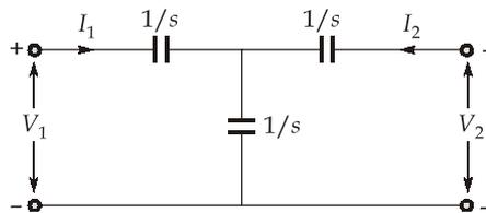
$$y_{11} = \left. \frac{I_1}{V_1} \right|_{V_2=0}$$
