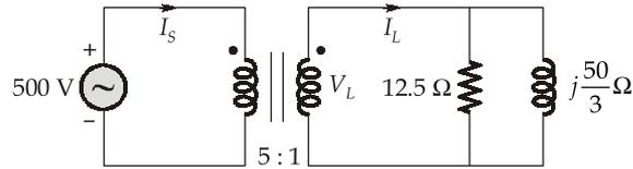
The load voltage,  $V_L = \frac{1}{5} \times 500 = 100 \text{ V}$
