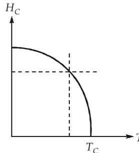
Where,  $T_C$  : Critical temperature ;  $H_C$  : Critical magnetic field
