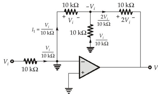
From, the diagram it is clear that  $V_0 = -2V_i - V_i = -3V_i$
