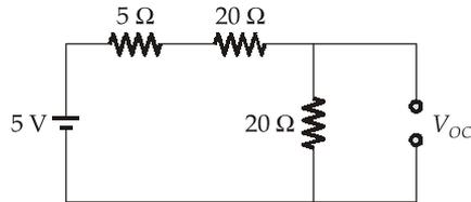
$$V_{OC} = 5 \times \frac{20}{20 + 25} = 2.22 \text{ V}$$
