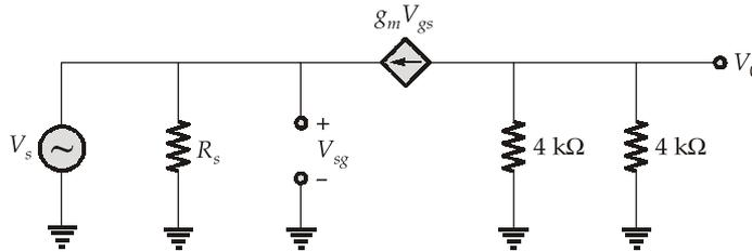
$$V_0 = -g_m V_{gs} (4 \text{ k}\Omega \parallel 4 \text{ k}\Omega)$$
